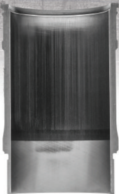
Severely Scuffed Liner After 44 Hours of Testing
